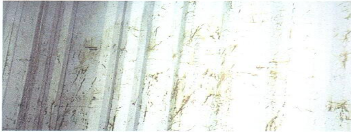
CONDITION PHOTO 6.39 /Scratches due to cargo loading that would not be acceptable to a shipper or lessee for shipment of dry-van general cargo, but would be acceptable for open-top cargo.
