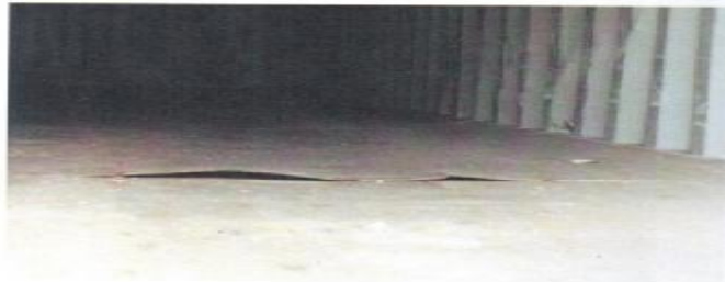
Photo 4.4 Delaminated plywood board, without indication of either impact or overloading and without breakage of an outer veneer. This is a wear item.
