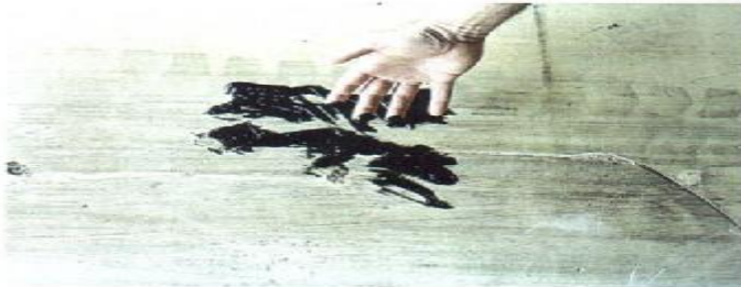
CONDITION PHOTO 6.17/Tar stain that would damage cargo and impede the safe loading and operation of the container.
