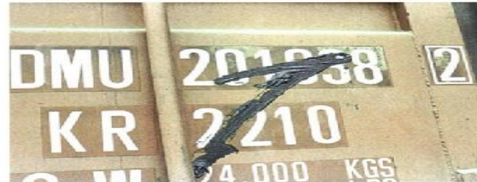
CONDITION PHOTO 6.74/Spillage on exterior that renders ISO markings illegible and would not be acceptable for shipment of dry-van cargo.
