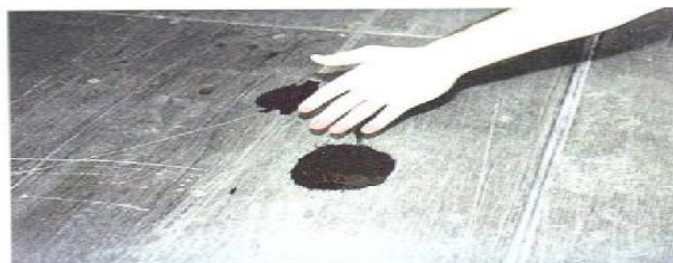
CONDITION PHOTO 6.16 /Pooled oil on floor surface that would damage cargo and impede the safe loading and operation of the container.
