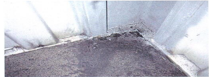
CONDITION PHOTO 6.30/Transferable burn marks on floor that could damage dry-van general cargo and are not acceptable to shippers or lessees for dry-vans.
