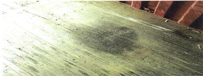
CONDITION PHOTO 6.9/Dry dust covering floor stains in an amount greater than would normally remain after a sweep out, and that would not be acceptable to the shipper or lessee.
