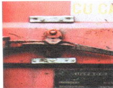
REPAIR NOT REQUIRED Bent door handle does not impair door operation or securement.
