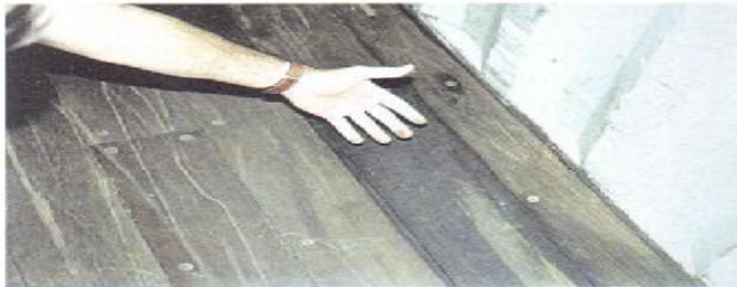
CONDITION PHOTO 6.13 /Damp oil stain that is transferable and that would damage dry-van general cargo.
