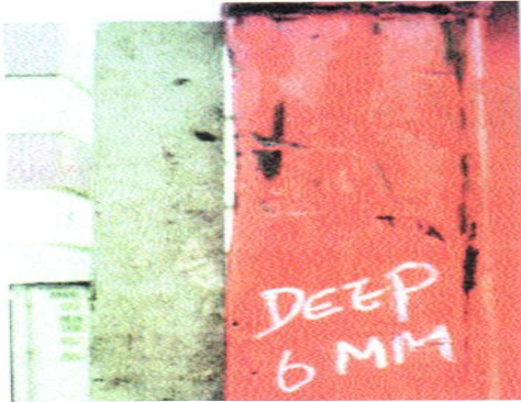
REPAIR NOT REQUIRED Corner post not dented in excess of 25 mm (1 in).
